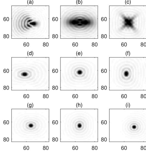
**Fig 9** Example of Fourier transforms of subimages used in processing, showing aberrations of peak; (a)  $\tilde{s}_\alpha$ , (b)  $\tilde{s}_\alpha^{(x)}$ , (c)  $\tilde{s}_\alpha^{(y)}$ , (d)  $\tilde{s}_\alpha^{(xx)}$ , (e)  $\tilde{s}_\alpha^{(xy)}$ , (f)  $\tilde{s}_\alpha^{(yy)}$ , (g)  $\delta_\alpha^{(x)} \tilde{s}_\alpha^{(x)}$ , (h)  $\delta_\alpha^{(y)} \tilde{s}_\alpha^{(y)}$ , (i)  $\delta_\alpha \tilde{s}_\alpha$ .
