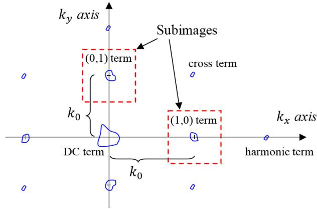
**Fig 5** Example of  $\tilde{s}(k_x, k_y)$ , two-dimensional spatial Fourier transform of sensor image, depicting locations of subimage selection about harmonic terms of interest.
