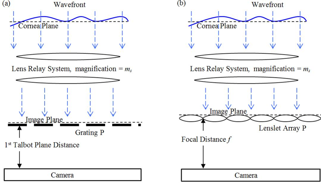
**Fig 3** Wavefront sensor: (a) employing grating with pitch  $P$  at appropriate distance from a camera to utilize Talbot effect, and (b) employing lenslet array with pitch  $P$  at appropriate distance from camera to produce focused spot pattern.
