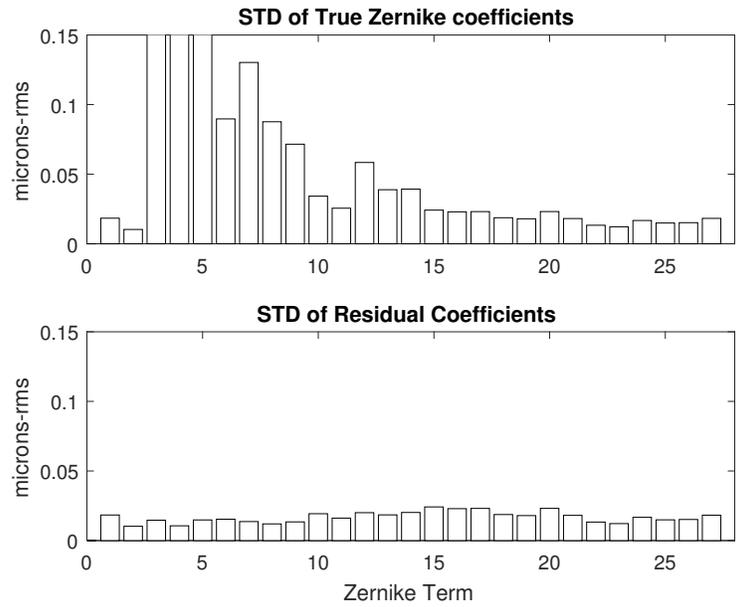
**Fig 12** Standard deviations of coefficients for each Zernike term in simulated data (top) and in residual error after estimate (bottom). Standard deviations of true Zernike coefficients 3, 4, and 5, are 0.27, 1.40, and 0.4274, respectively.
