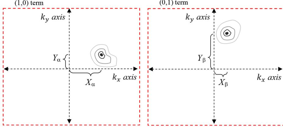
**Fig 6** Subimages  $\tilde{s}_\alpha$  and  $\tilde{s}_\beta$  extracted from Fig. 5, depicting peak locations resulting from aberrations.
