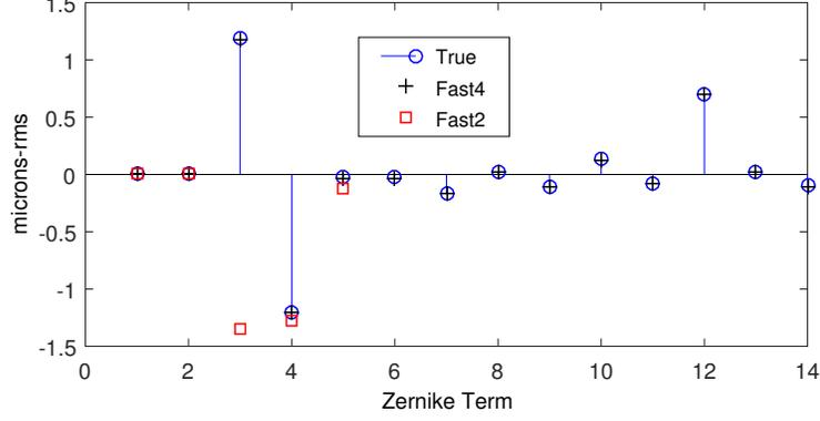
**Fig 8** True Zernike coefficients used in simulation, and result of algorithm to estimate 4th order Zernikes (Fast4), as well as a version that stops after estimating 2nd order coefficients (Fast2). Net rms error (the root of the sum of the errors for each coefficient squared) is 0.043 microns-rms for Fast4, and 2.65 microns-rms for Fast2.
