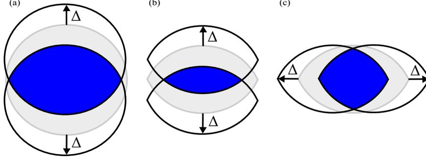
**Fig 7** An excessively large  $\Delta$  parameter reduces the amount of pupil information utilized, (a) by  $2\Delta$  for the first product  $s^{(y)}$  (and similar for  $s^{(x)}$ ), (b) by  $4\Delta$  for the second products  $s^{(yy)}$  (and similar for  $s^{(xx)}$ ), and (c) by  $2\Delta$  in both directions for the remaining second product  $s^{(xy)}$ . So a smaller  $\Delta$  is desirable to retain the most pupil area.
