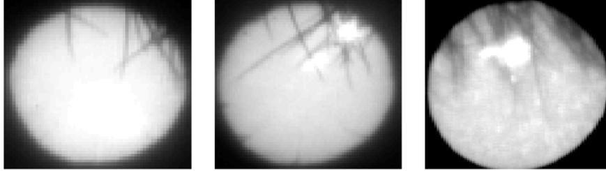
**Fig 2** Examples of eyelash shadows partly occluding pupil signal; the bright regions are reflections of the laser source from the cornea and subsequent structures.
