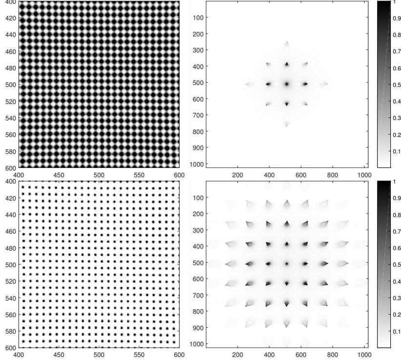
**Fig 4** Simulated grating (top row) and Shack-Hartmann (bottom row) result; detector image (left) and spatial-frequency image (right). Detector images are 1024x1024 pixels covering 10 millimeters, with a pitch of 42 microns and a magnification of 2.0; here images are zoomed to central 200x200 pixel region for visibility of pattern.
