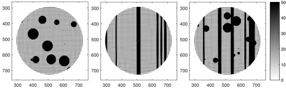
**Fig 10** Image artifact examples, with random spots or lines to demonstrate algorithm robustness.
